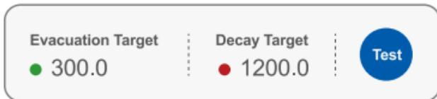
Setting the Decay target and conducting a leak test can help you judge the sealing condition of the system!
