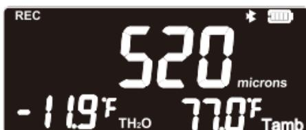
The device can only display two temperature values when used offline.
